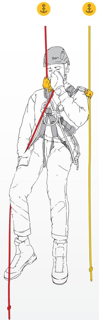
The use of a sling or lanyard when creating the anchor point. The anchor point must have min. strength 24 kN.
